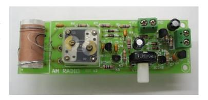
The second component of the TRF is the coil & ferrite bar. We supply the coil prewound with 90 turns of 3 strand Litz wire. We got these coils from a commercial manufacturer of these coils who supplies exactly the same item to AM radio manufacturers. Litz wire consists of many strands of fine enamelled wire twisted together with cotton to add strength. Litz wire has a significantly lower resistance to RF than a single wire and is used in virtually all commercial coils.
